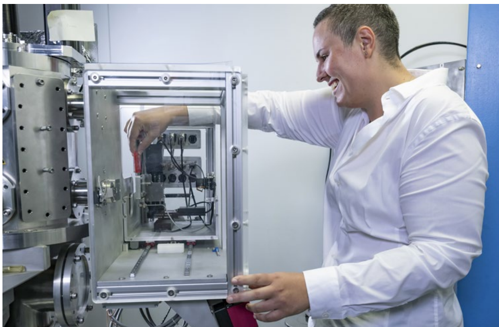
Dr Ferlazzo placing a biological sample holder into a vacuum beam irradiation chamber.
