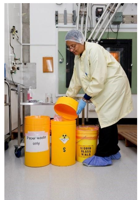
Right: Sorting low level waste into containers
