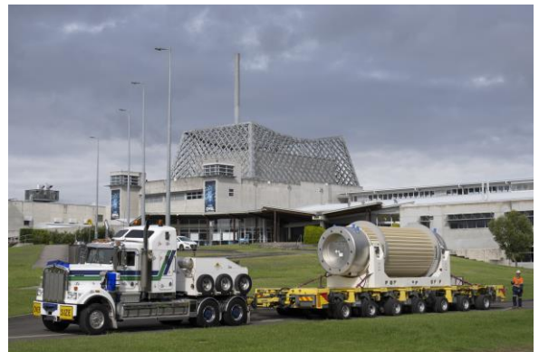
Left: A TN-81 canister of intermediate level waste being offloaded from the ship, ready for loading onto the truck.
