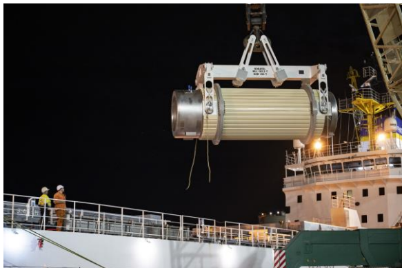
Left: A TN-81 canister of intermediate level waste being offloaded from the ship, ready for loading onto the truck.
