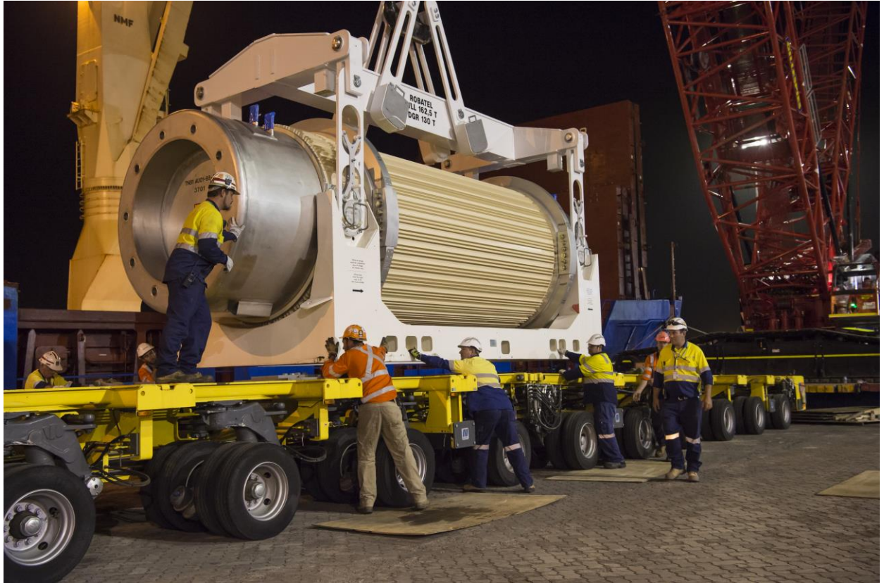
Above: A TN-81 canister of intermediate level waste being loaded onto a truck for return to ANSTO's Lucas Heights for interim storage.
