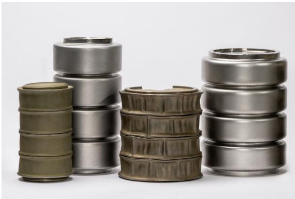
Left: ANSTO Synroc® canisters pre and post the hot isotopic pressing process, and Right: ANSTO Synroc® canister ready for hot isotopic pressing
