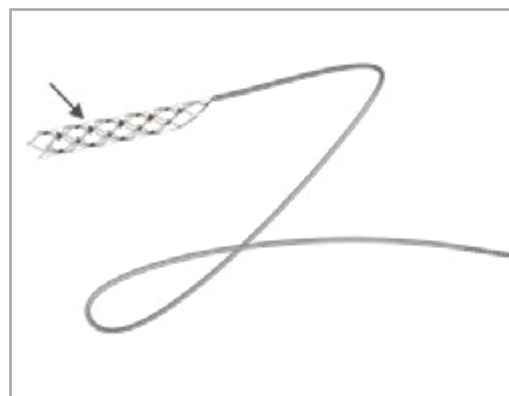
FIGURE 1: Image of the Stentrode™ in its expanded form, showing the electrodes (arrow) which are 8 x 750 micrometres (µm) in size.
