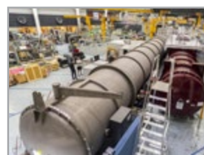
Small Angle Neutron Scattering (SANS) instruments Quokka (left) and Bilby (right) at ANSTO used to quantify the nanoscale precipitation in structural alloys.
