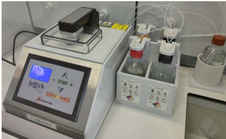
Figure 10 Nisene JetEtch Pro CuProtect installed within a fume cupboard
