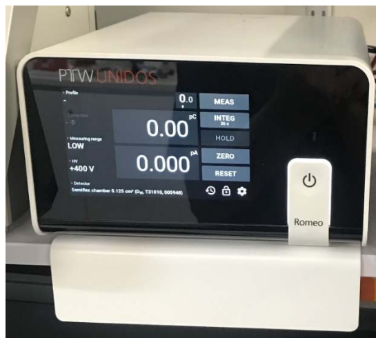
Figure 7 The PTW UNIDOS Romeo electrometer provides accurate dose rate measurements of the photon beams
