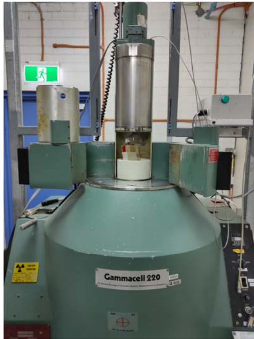
Figure 3 Gammacell 220 gamma irradiation tank
