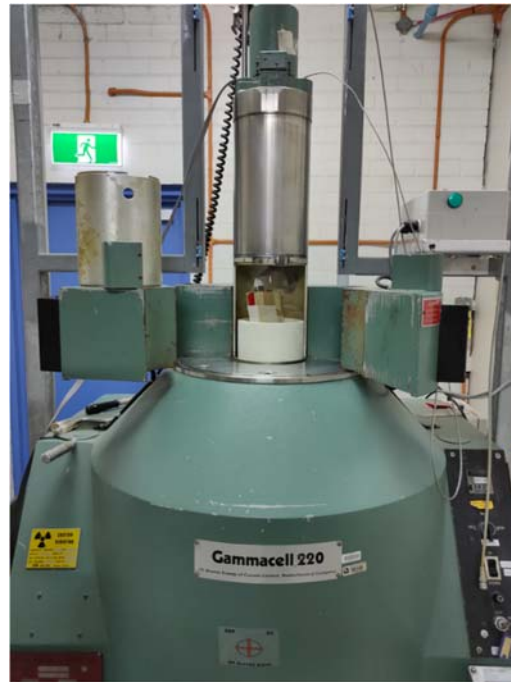
Figure 3 Gammacell 220 gamma irradiation tank
