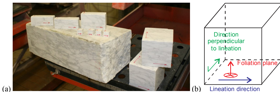
Fig. 2. (a) Samples of Carrara marble and (b) their geological framework. The larger cube-like marble samples measure 100 mm on side.
