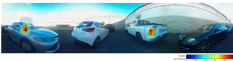
Checkpoint search where multiple vehicles can be screened in a single acquisition. The panorama shows the location of two hidden 137 Cs sources of radiation.
