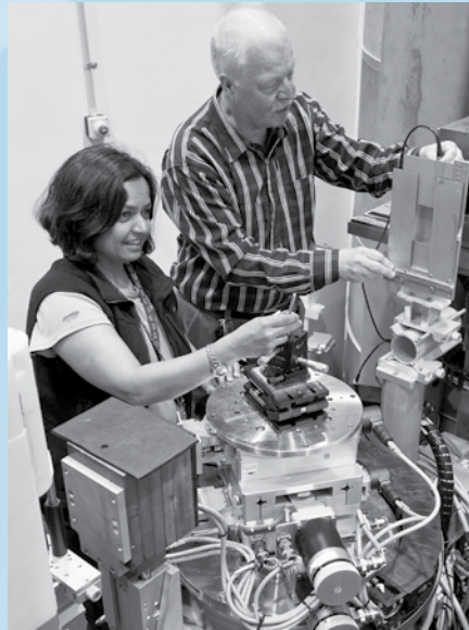
Mohana Yethiraj (left) and Sergey Danilkin (right) working on ANSTO's triple-axis spectrometer, Taipan.
