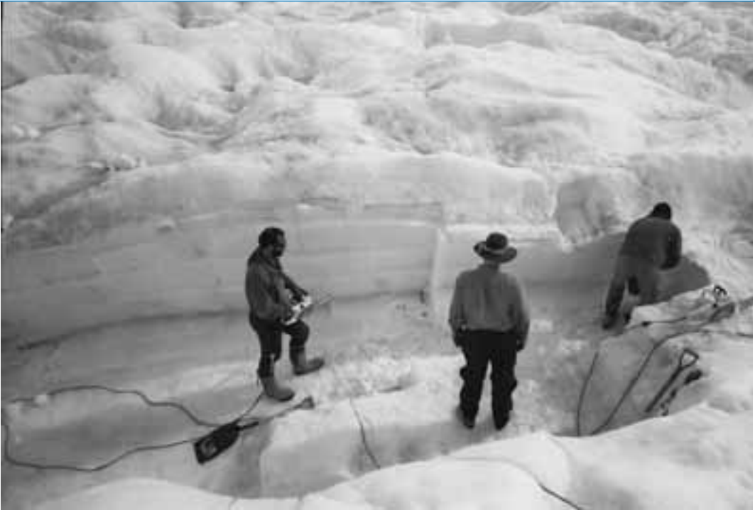
Mining 12,000-year-old ice on the ice margin in Greenland. The team melted 15 tonnes of ice, collecting the ancient air trapped within and separating the methane for analysis. Photo courtesy Dr Vas Petrenko.
