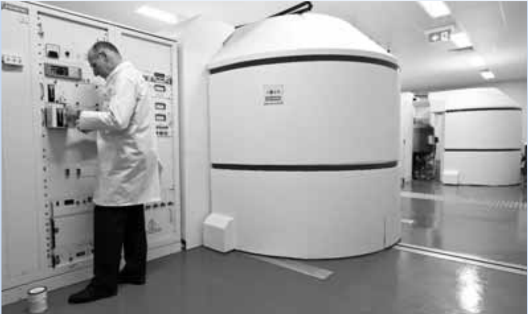
The two PETNET mini-cyclotrons will produce a short-lived glucose radiopharmaceutical used in positron emission tomography (PET) scanning.
