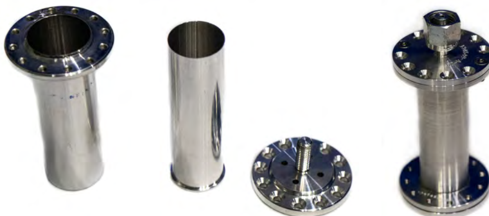
Figure 6.23: Photo of (from left to right) an aluminium annular can outer cup, inner cup, lid, and an assembled a gas delivery can.
