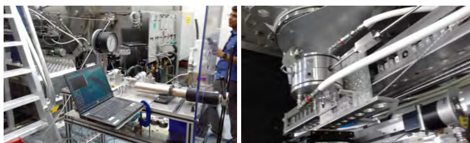
Figure 4.7: Photo of SPC-1 on Quokka (right) and pressure intensifier(left).
