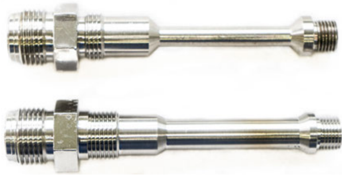
Figure 6.31: Photo of 7 mm (top) and 10 mm (bottom) stainless steel cans for high pressure furnace experiments.
