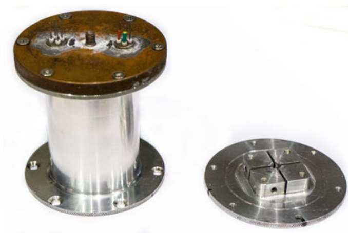
Figure 6.33: Photo of exchange gas can for bottom-loading cryofurnaces.
