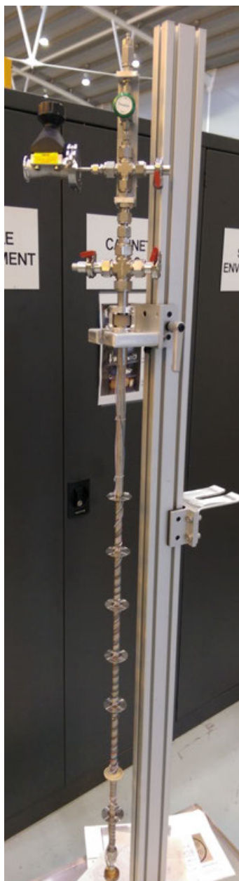
Figure 6.18: Version 1 gas delivery stick
