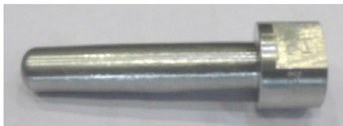
Figure 6.29: Photo of an aluminium can for clathrate samples.
