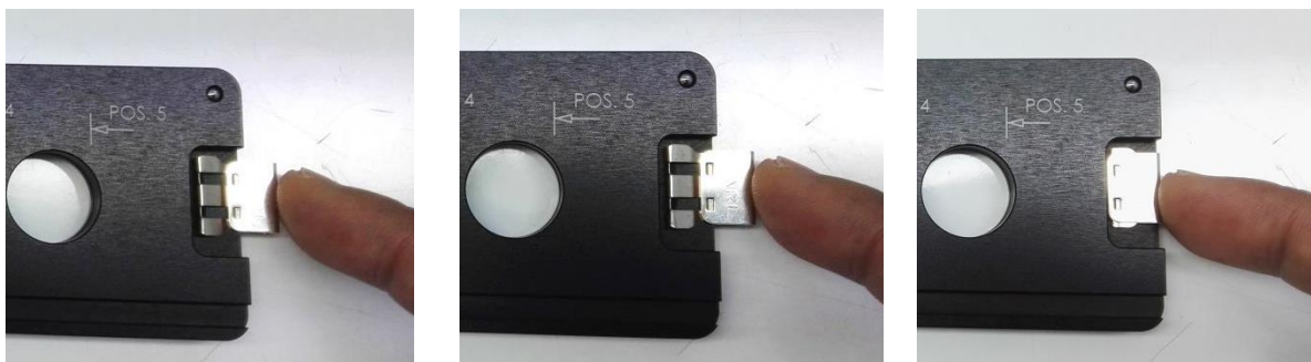
Figure 28. Image showing the use of the spring clip to secure the two components of the sample holder together.
