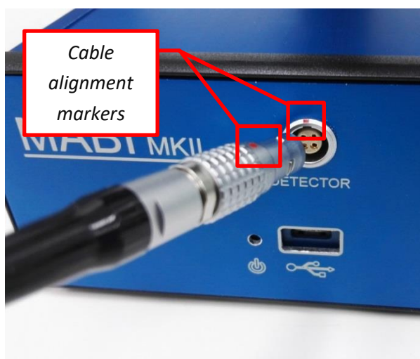
Figure 3. Images of the photo-detector and USB cable installation.
