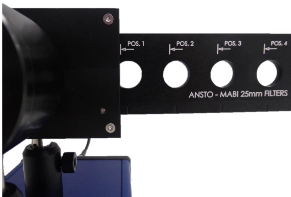
Figure 29. Image of the filter holder correctly aligned to position 1 (POS. 1).
