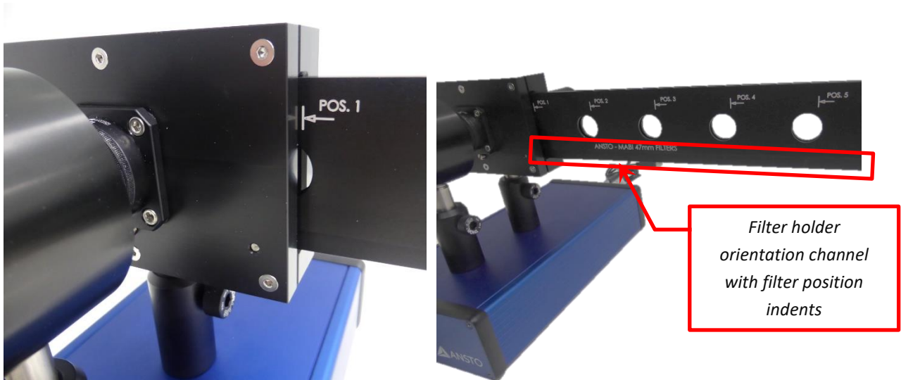
Figure 20. These pictures show the correct alignment of position 1 marker on the 25mm diameter filter holder with the sample holder edge. Similar alignment can be performed for position markers 2 to 8. Note: there is an orientation channel on the bottom edge of each filter holder to ensure the filter holder can only be inserted in the correct orientation. Ball detent notches along the orientation channel also provide physical feedback as each filter position is correctly aligned during holder insertion.
