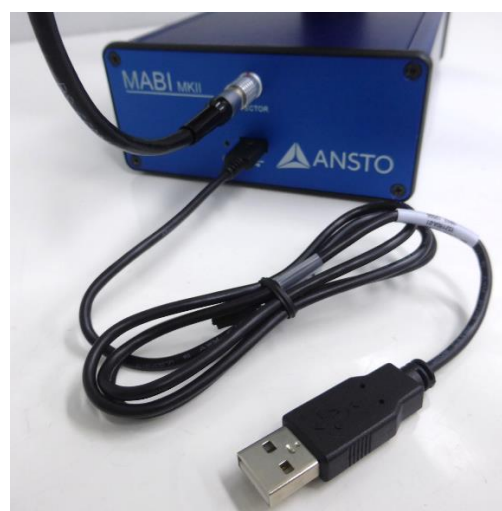
Figure 3. Images of the photo-detector and USB cable installation.
