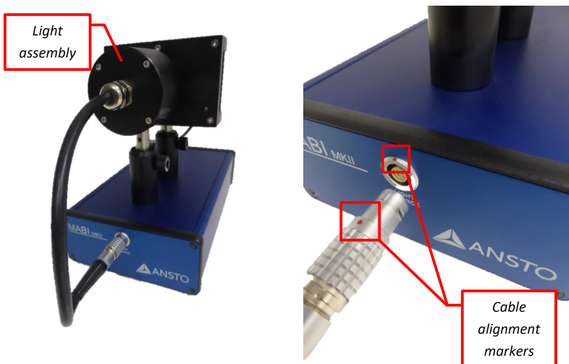
Figure 2. Images of the light assembly cable installation.
