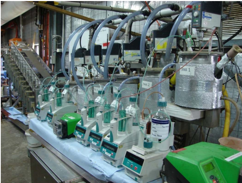
Figure B2 Mixed rare earths carbonate precipitation circuit at ANSTO
