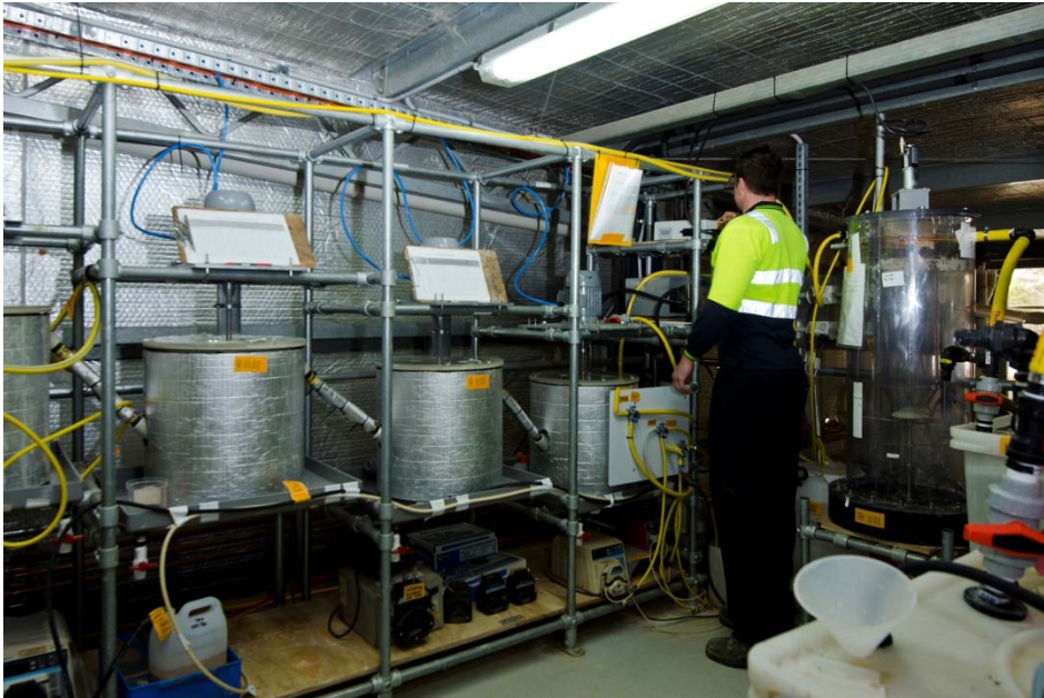
Figure B1 Rare earths leach circuit – pH controlled acid leach – at ANSTO
