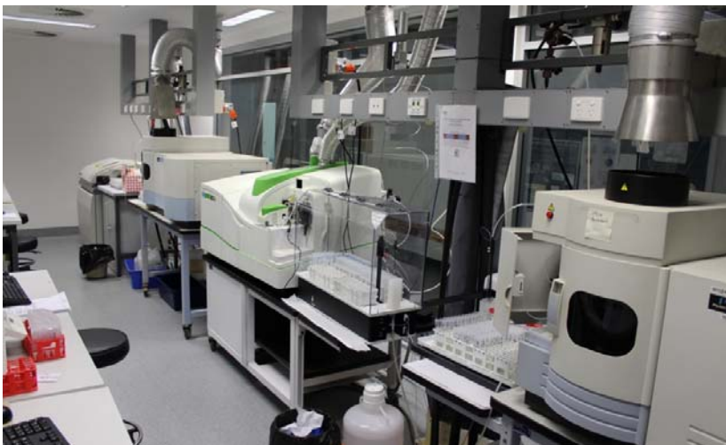
Figure G3 Inductively Coupled Plasma Optical Emission and Mass Spectrometers (ICP-OES x 2 and ICP-MS x 2)
