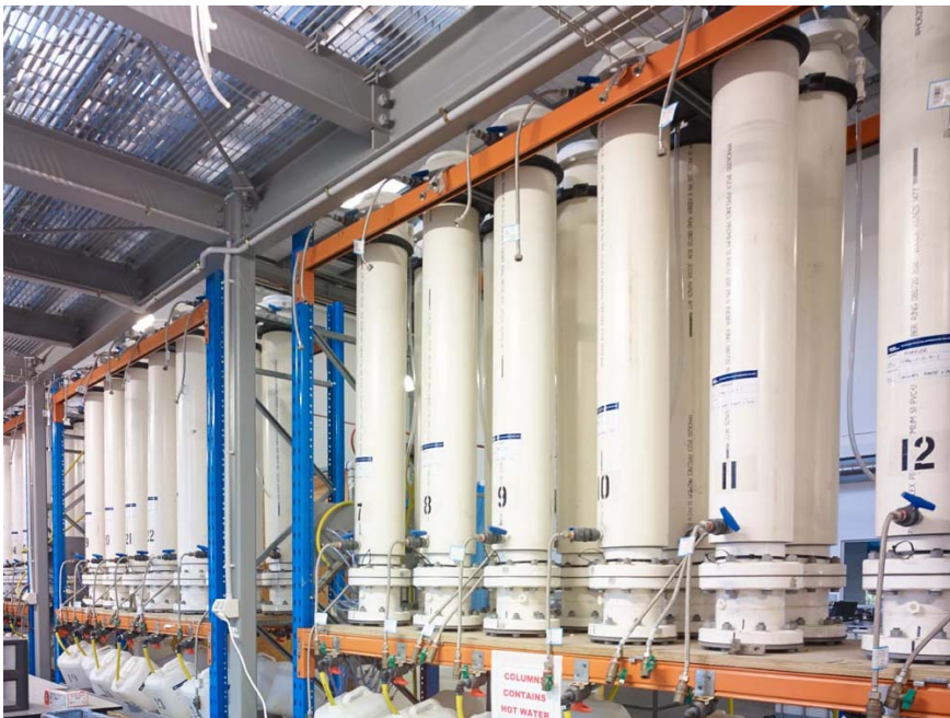
Figure A7 Heap leach column test rig (2 m) designed / built by and installed at ANSTO. 4 m variants also available.
