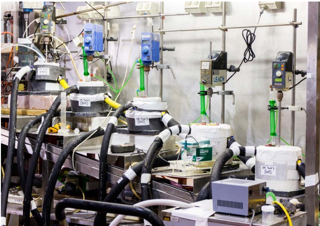
Figure C4 Lithium carbonate precipitation circuit at ANSTO
