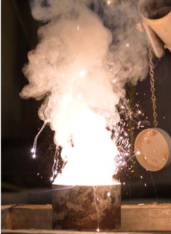
Figure D3 Ferro-niobium production - ~200 g button scale
