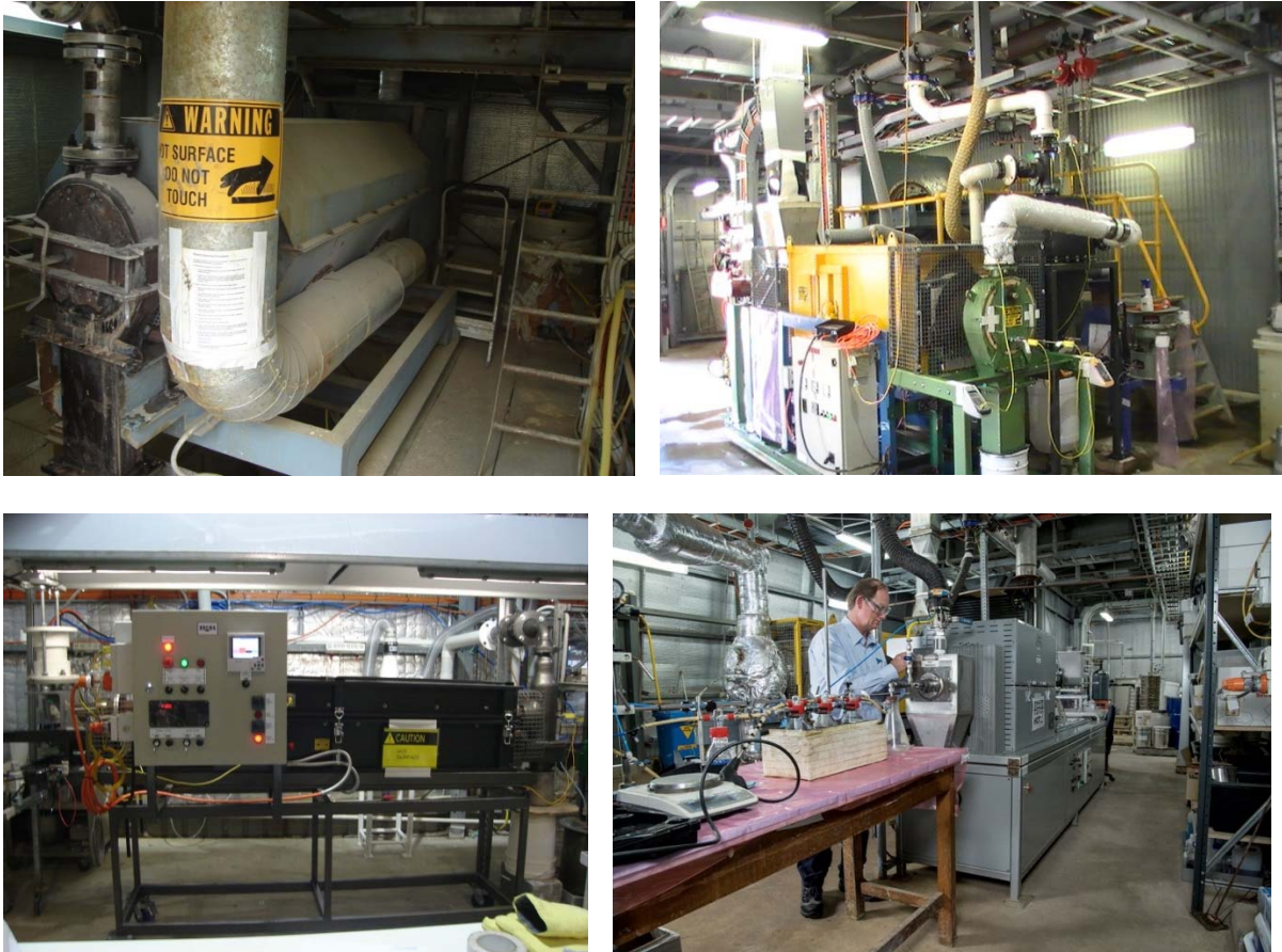
Figure B7 Kilns for sulphation roasting as part of RE processing – throughput rates ranging from 100s' kg/h (top left), to 10s' kg/h (top right), to ~2 kg/h (bottom right), and <1 kg/h (bottom right) – installed at ANSTO
