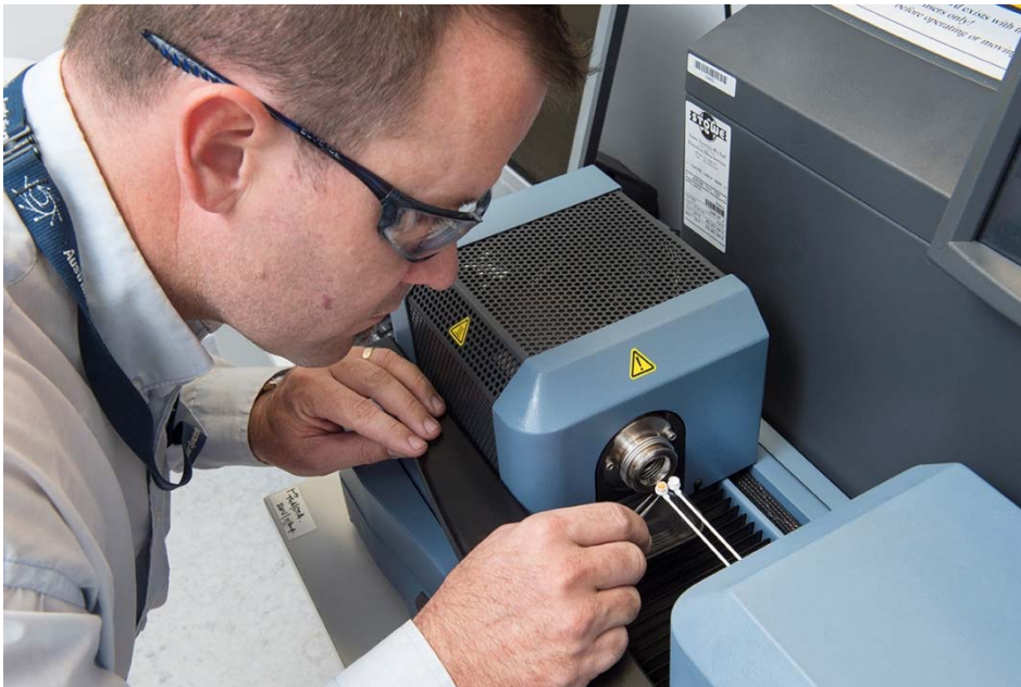
Figure G6 Thermogravimetric Analysis and Differential Scanning Calorimetry (TGA-DSC)
