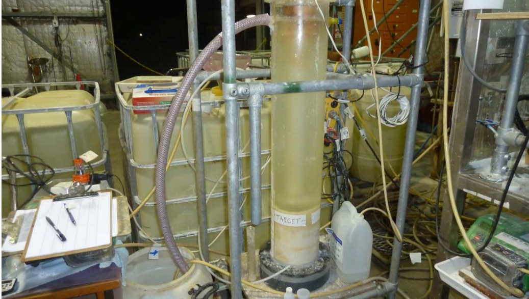
Figure C3 Softening circuit for lithium processing at ANSTO
