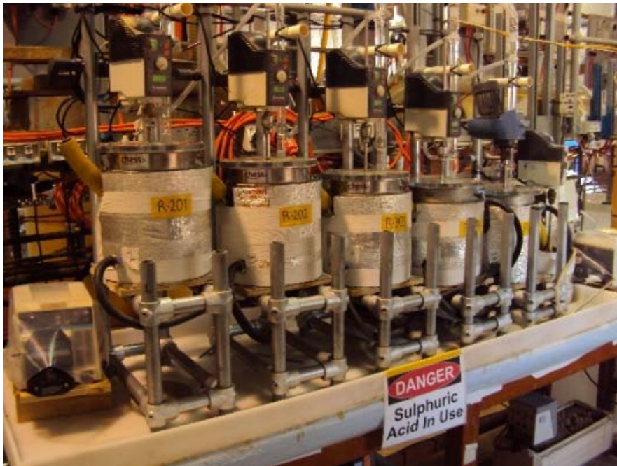
Figure C1 Lithium ore leach circuit at ANSTO
