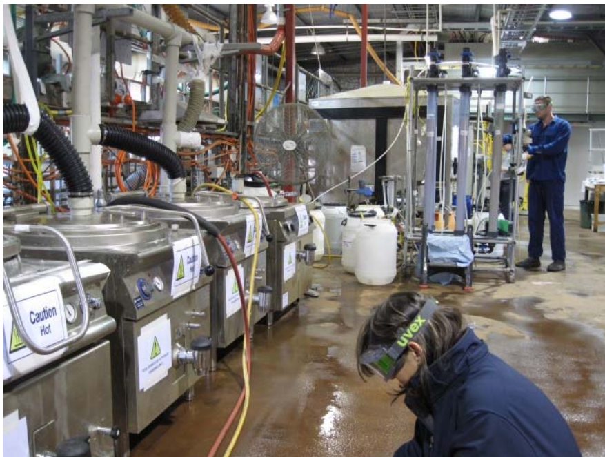
Figure C2 Evaporation and Ca / Mg IX circuits at ANSTO. Up to 20 L/h per unit
