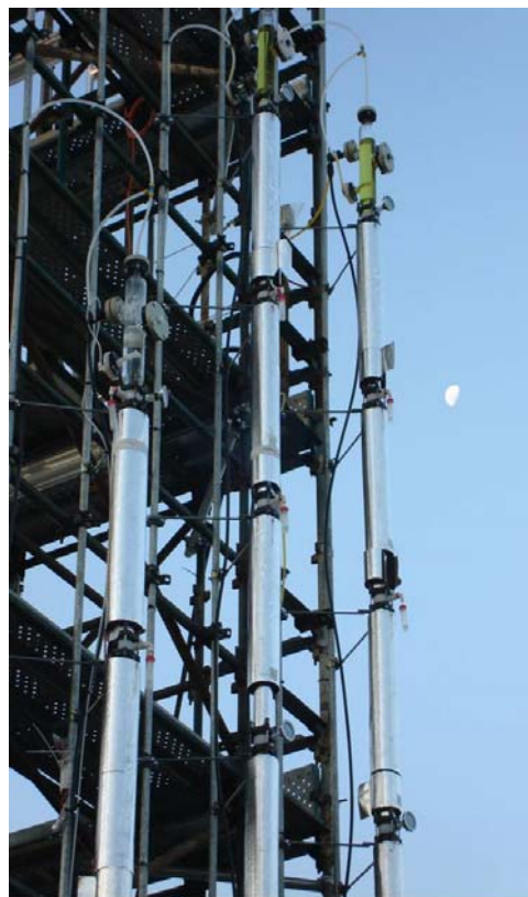
Figure H3 Pulsed column demonstration plant designed / built by ANSTO for uranium at ANSTO
