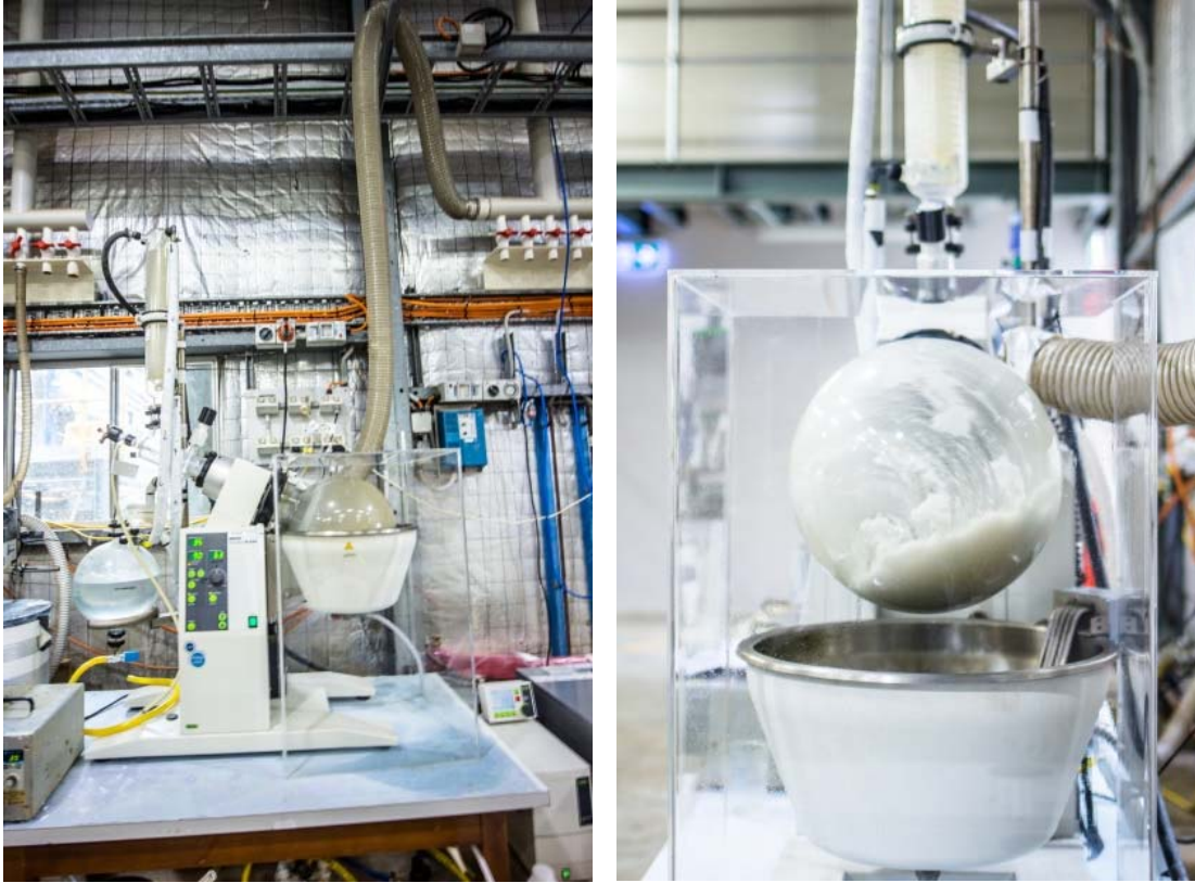
Figure C5 Lithium sulphate crystalliser – ~2 kg per batch – semi-continuous
