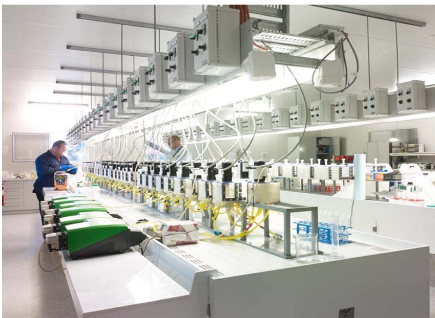
Figure H1 State-of-the-art SX mini-plant pilot facilities for small scale, continuous testing – modular design for limitless circuit configurations at ANSTO
