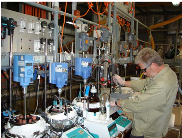
Figure A4 Uranium leach circuit – pH controlled acid leach at ANSTO
