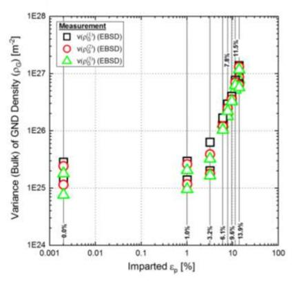
$\Rightarrow$  The development of the **variance** of GND density distribution as a function of imparted plastic strain  $(\epsilon_p)$  for all tested specimens.
