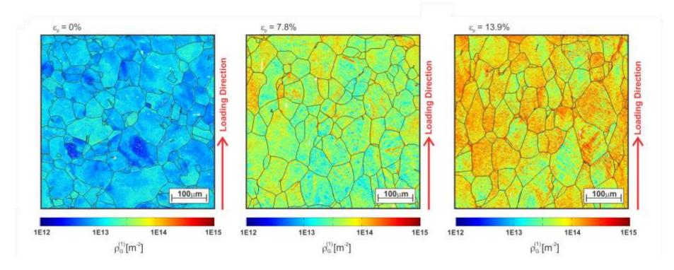
$\Rightarrow$  Density of geometrically-necessary dislocations (GND,  $\rho_G$ ) maps calculated from the EBSD-measured Euler Angles ( $\phi_1$ , $\Phi$ , $\phi_2$ ) for specimens with 0% (as-received), 7.8% and 13.9% of imparted plastic strain.
