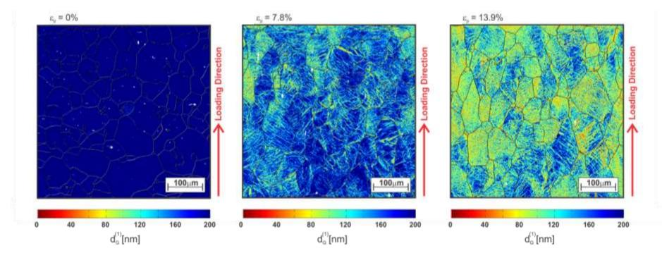
$\Rightarrow$  Spacing between geometrically-necessary dislocations (GND, d<sub>G</sub>) recalculated from the GND density ( $\rho_G$ ) for specimens with 0% (as-received), 7.8% and 13.9% of imparted plastic strain.
