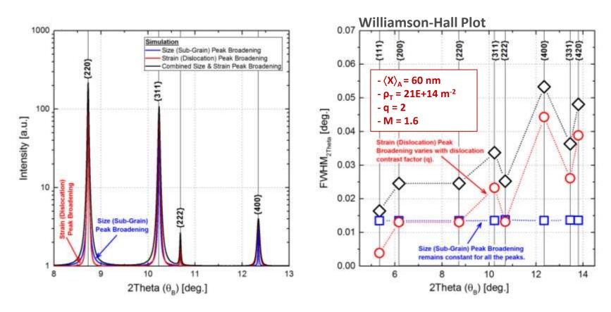
⇒ The broadening due to the size of the coherently diffracting domains (sub-grains) is the same for all hkl diffraction peaks, while the broadening component due to the strain field of present dislocations varies between diffraction peaks. This variation in the strain (dislocation) broadening is not monotonous due to the anisotropic behaviour described by the dislocation contrast factors.
