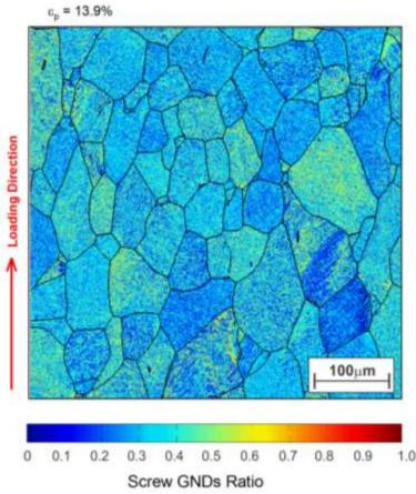
$\Rightarrow$  Map showing the ratio of screw dislocations to the total number of dislocations in the solution (6) for the specimen with 13.9% imparted plastic strain.
