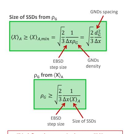
$\Rightarrow$  This defines the connection between EBSD-measured  $\rho_G$  and HRSD-measured  $\langle X \rangle_A$  one can then estimate  $\rho_G$  from  $\langle X \rangle_A$ .
