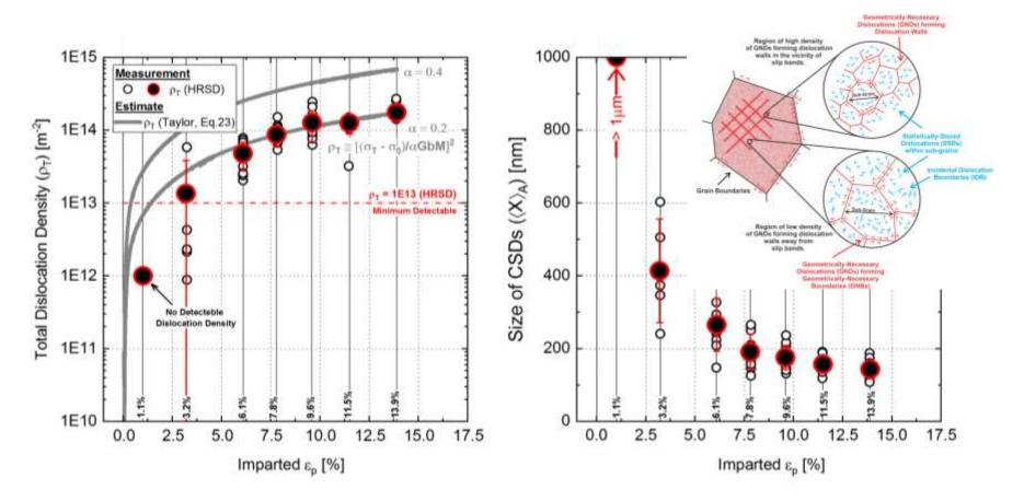
$\Rightarrow$  Total dislocation density ( $\rho_T$ ) and size of the coherently scattering domains (SCDs) obtained by line profile analysis (LPA) of HRSD patterns as a function of imparted plastic strain ( $\epsilon_p$ ) - open symbols represents individual measurements along the sample loading axis, and solid symbol represents the mean values.
