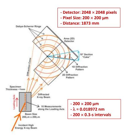
⇒ High-resolution synchrotron diffraction (HRSD) set-up at 1-ID high-energy beamline at the Advanced Photon Source (APS), Argonne National Laboratory (ANL).
