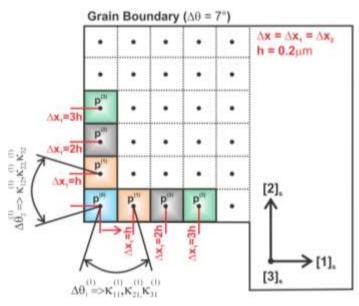
$\Rightarrow$  GNDs have a geometrical consequence giving rise to a curvature of the crystal lattice, which can be measured by EBSD technique. The crystal orientation  $(\phi_1, \Phi, \phi_2)$  changes only when the electron beam crosses an array of GNDs that has a net non-zero Burger's vector.
