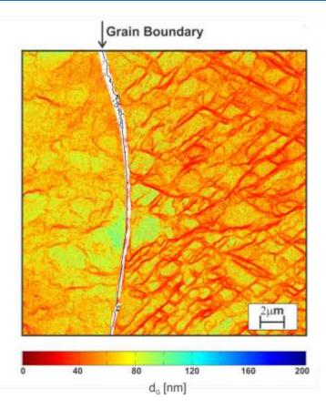
$\Rightarrow$  Spacing between geometrically-necessary dislocations (GND, d<sub>G</sub>) recalculated from the GND density ( $\rho_G$ ).
