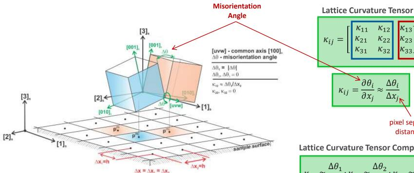
⇒ A schematic representation of lattice curvature components calculation between two neighbouring crystals misoriented ( $\Delta\theta$ ) by a rotation around the common crystallographic axis [100], ([uvw],) and separated by pixel separation distance ( $\Delta x_2$ ). Note, that in this example:  $\kappa_{12} \approx \Delta \theta_1 / \Delta x_2$ , and  $\kappa_{22}, \kappa_{32} = 0$ .
