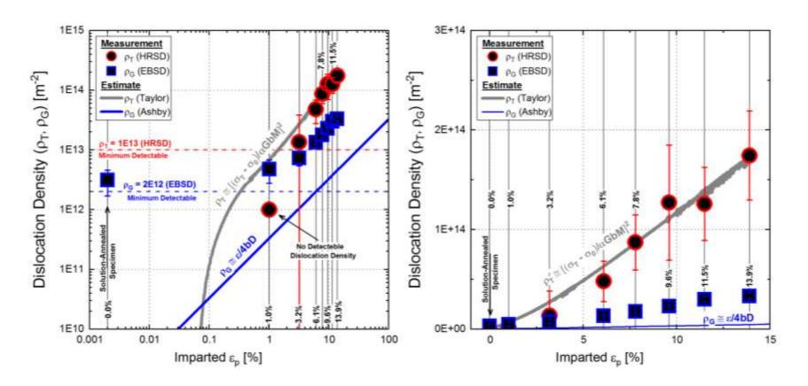
$\Rightarrow$  Comparison of the HRND-measured total dislocation density ( $\rho_T$ ) and the EBSD-measured density of GNDs ( $\rho_G$ ), together with expected dislocation densities calculated using the modified Taylor's model, and single-slip Ashby's model.
