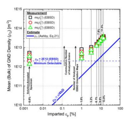
$\Rightarrow$  The development of the **mean** GND density distribution as a function of imparted plastic strain  $(\epsilon_p)$  for all tested specimens.
