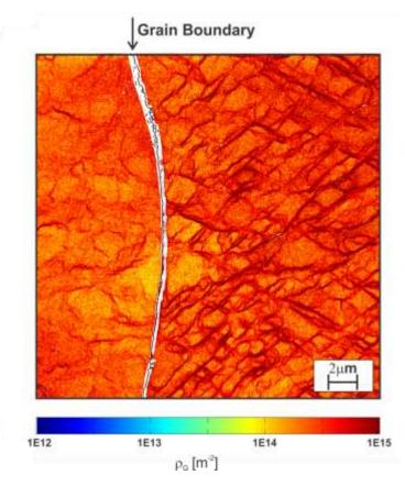
$\Rightarrow$  Density of geometrically-necessary dislocations (GND,  $\rho_G$ ) calculated from the EBSD-measured Euler Angles  $(\phi_1, \Phi, \phi_2)$ .
