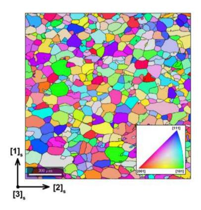
⇒ EBSD orientation map showing the overall equiaxed grain structure of our solution-annealed Ni201 before testing.
