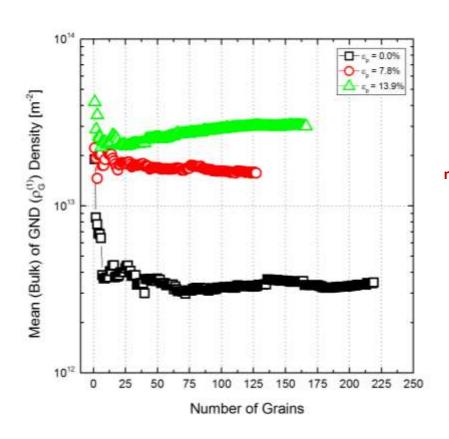
$\Rightarrow$  The development of the mean GND density as a function of number of analysed grains in GND density maps for specimen with 0% (as-received), 7.8% and 13.9% of imparted plastic strain  $(\epsilon_p).$
