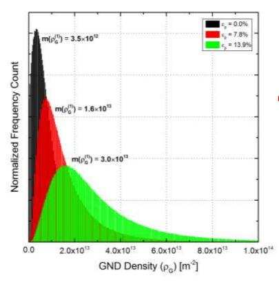
$\Rightarrow$  Distribution (histogram) of discrete GND density ( $\rho_G$ ) measurements for specimen with 0% (as-received), 7.8% and 13.9% of imparted plastic strain ( $\epsilon_p$ ).
