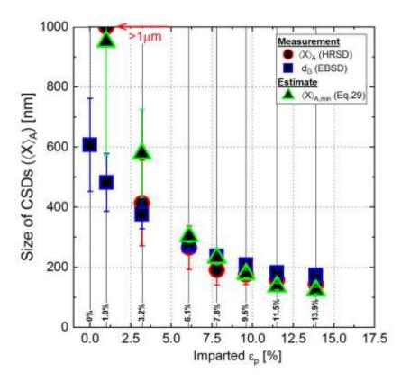
$\Rightarrow$  Comparison of the HRSD-measured size of CSDs (red circles) with EBSD-measured spacing of GNDs ( $d_G$ ) (blue squares), and the estimated minimum size of CSDs (green triangles) from EBSD-measured density of GNDs ( $\rho_G$ ).
