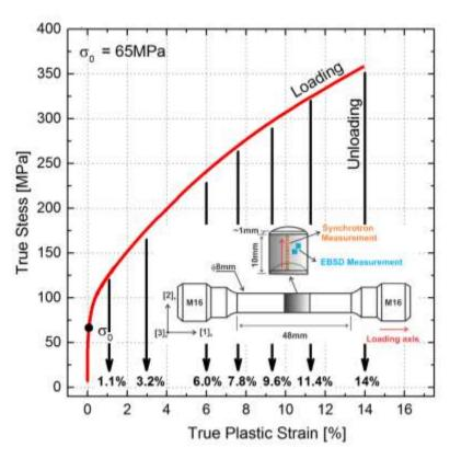
⇒ Interrupted tensile tests were performed to varying levels of imparted plastic strain. Samples were extracted from the gauge length for EBSD and HRSD measurement.
