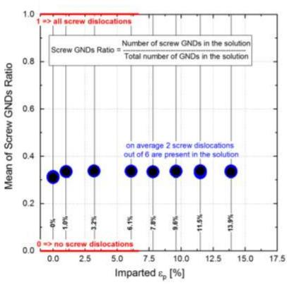
$\Rightarrow$  Screw dislocation ratio as a function of imparted plastic strain for all tested specimens.
