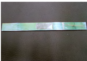
Figure 3b. Anton Paar platinum filament, with cavity
