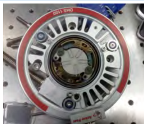
3c. The DHS1100 furnace showing the sample position. The sample/sample holder is held in place with clips.
