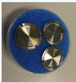
3e. DHS1100 powder sample holders. These are 20 mm in diameter and 1 mm deep.
