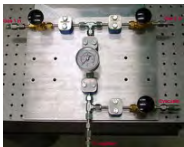
Figure 6. Gas mixing and evacuation manifold
