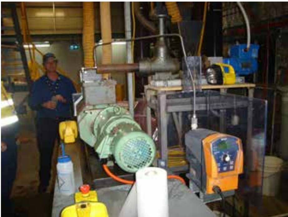
Figure B4 Twin-shaft pug mixer testing for acid / ore mixing / feeding at ANSTO
