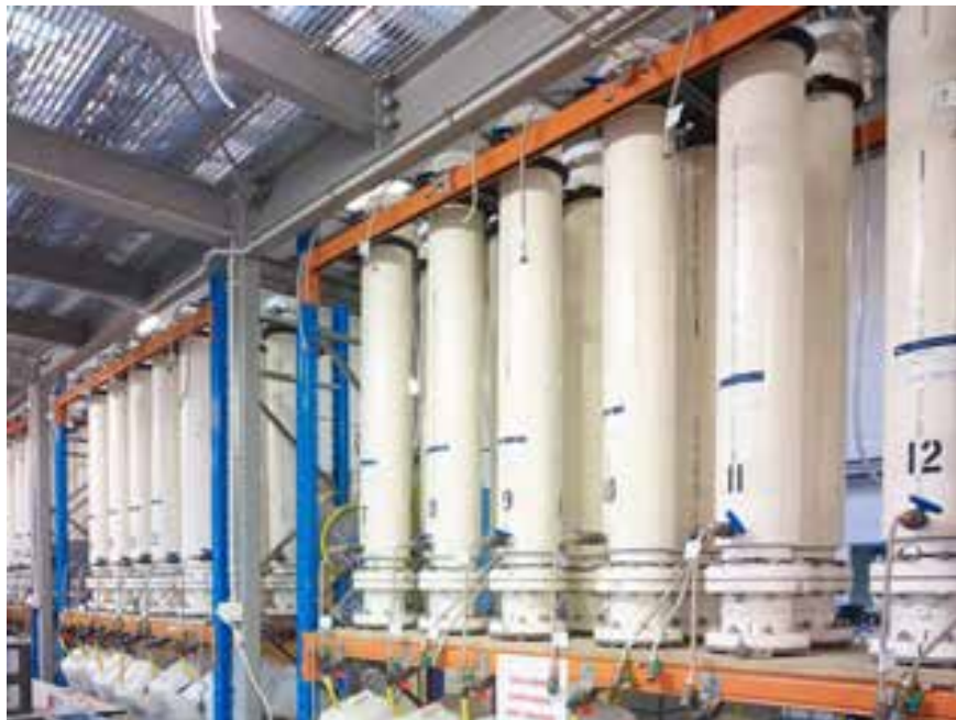
Figure A7 Heap leach column test rig (2 m) designed / built by ANSTO installed at ANSTO. 4 m variants also available.
