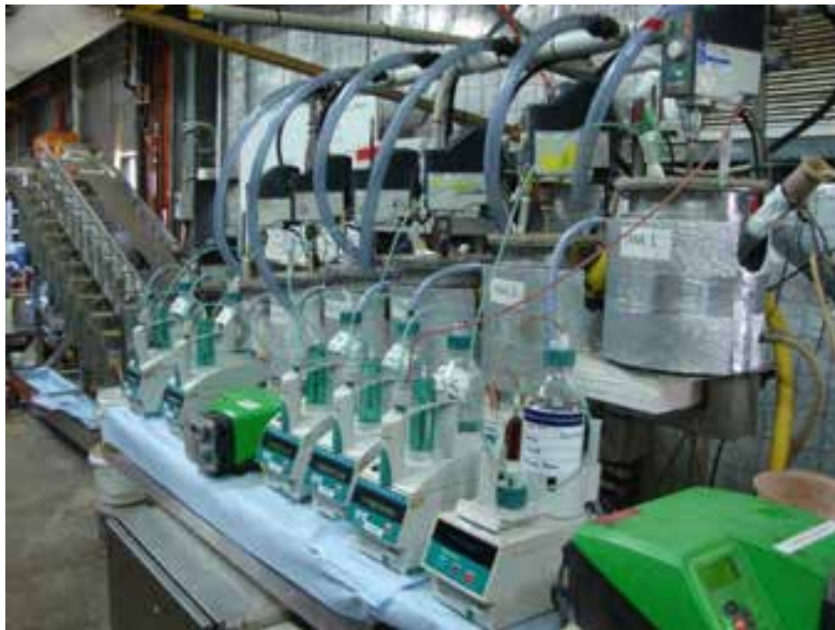
Figure B2 Mixed RE carbonate precipitation circuit at ANSTO
