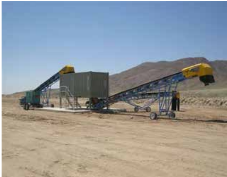
Figure A9 Ore sorter pilot plant trial managed and operated by ANSTO on site
