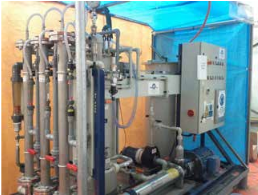
Figure A8 Nanofiltration continuous pilot rig installed at ANSTO
