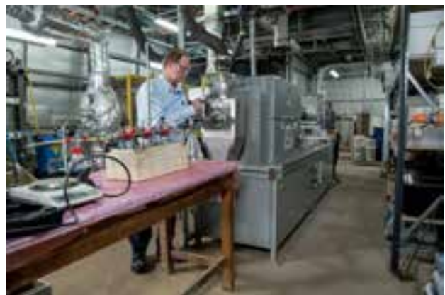
Figure B7 Kilns for sulphation roasting as part of RE processing – throughput rates ranging from 100s' kg/h (top left), to 10s' kg/h (top right), to ~2 kg/h (bottom right), and <1 kg/h (bottom right) – installed at ANSTO
