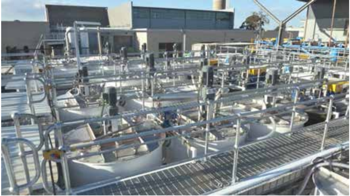
Figure C9 Brine processing demonstration plant at ANSTO – impurity removal circuit
