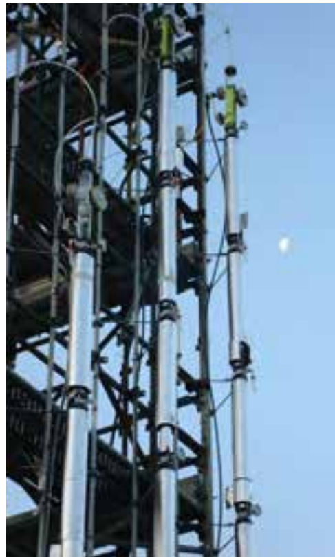
Figure H3 Pulsed column demonstration plant designed / built by ANSTO for uranium at ANSTO
