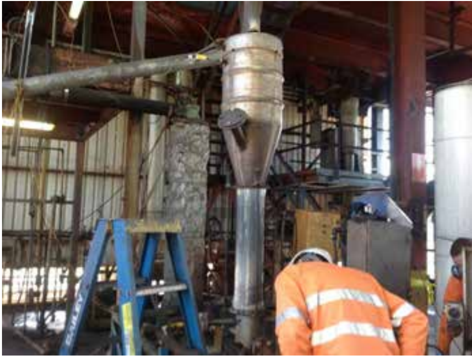
Figure B5 Fluidised bed testing for acid / ore drying / agglomeration on site
