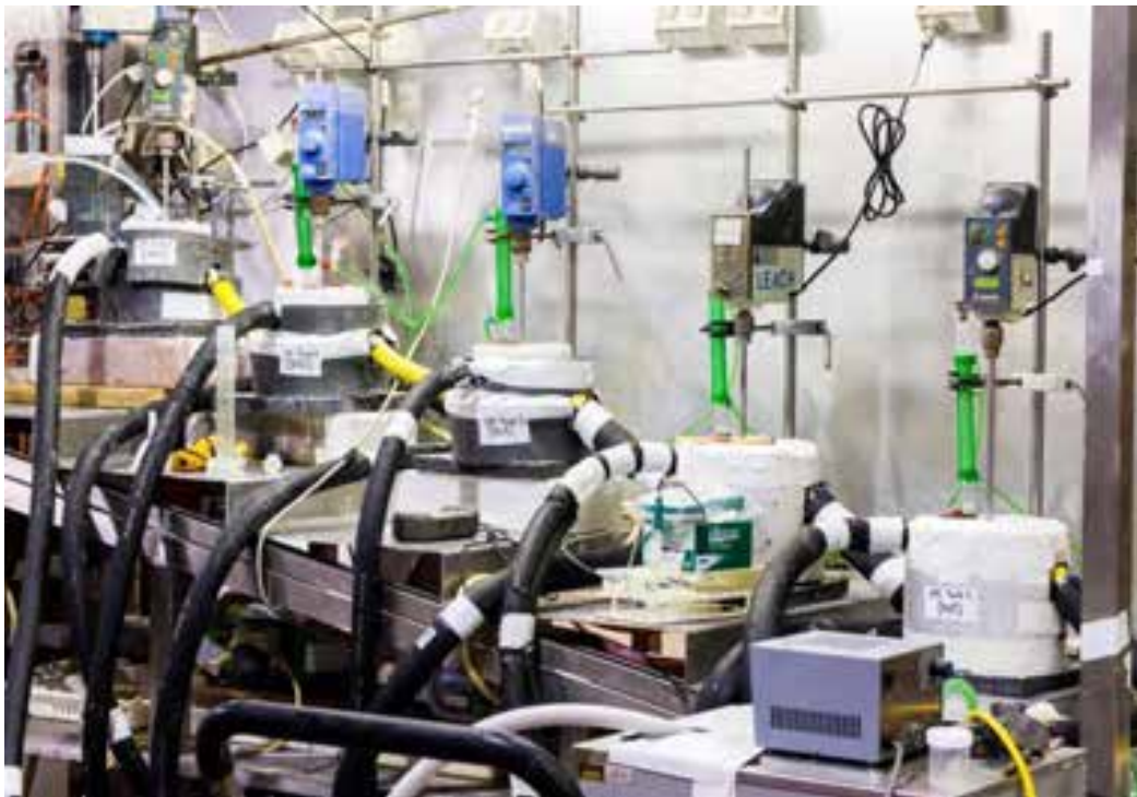
Figure C4 Lithium carbonate precipitation circuit at ANSTO
