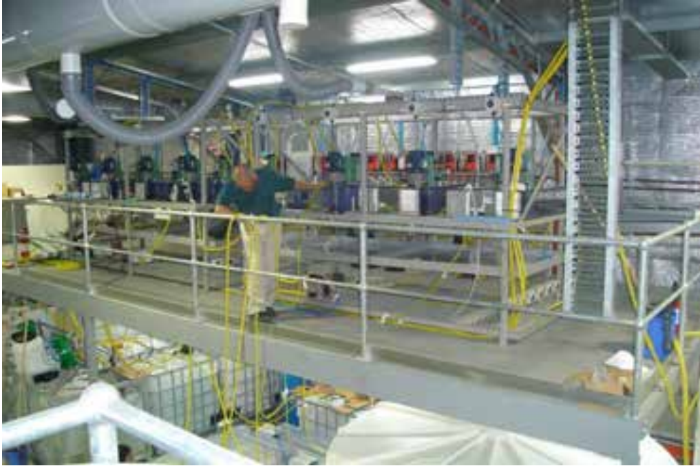
Figure H2 SX demonstration plant designed / built by ANSTO for zirconium at ANSTO
