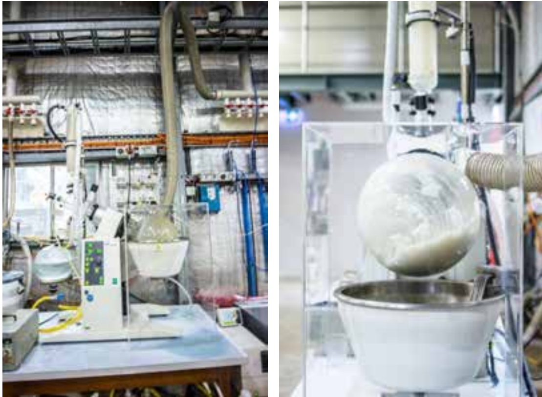
Figure C5 Lithium sulphate crystalliser – ~2 kg per batch – semi-continuous
