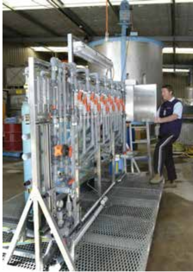
Figure A3 Fixed bed IX rig designed / built by ANSTO installed at ANSTO
