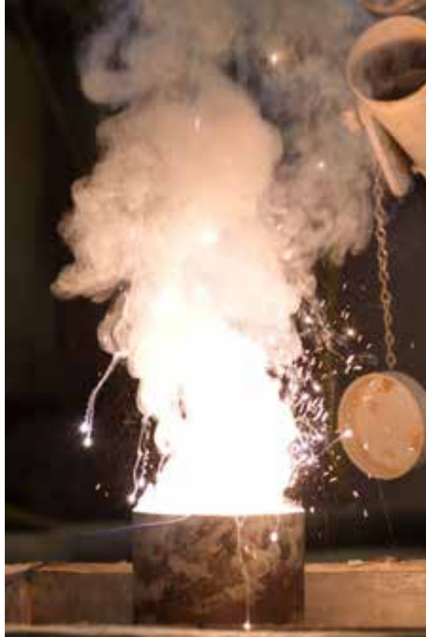
Figure D3 Ferro-niobium production - ~200 g button scale
