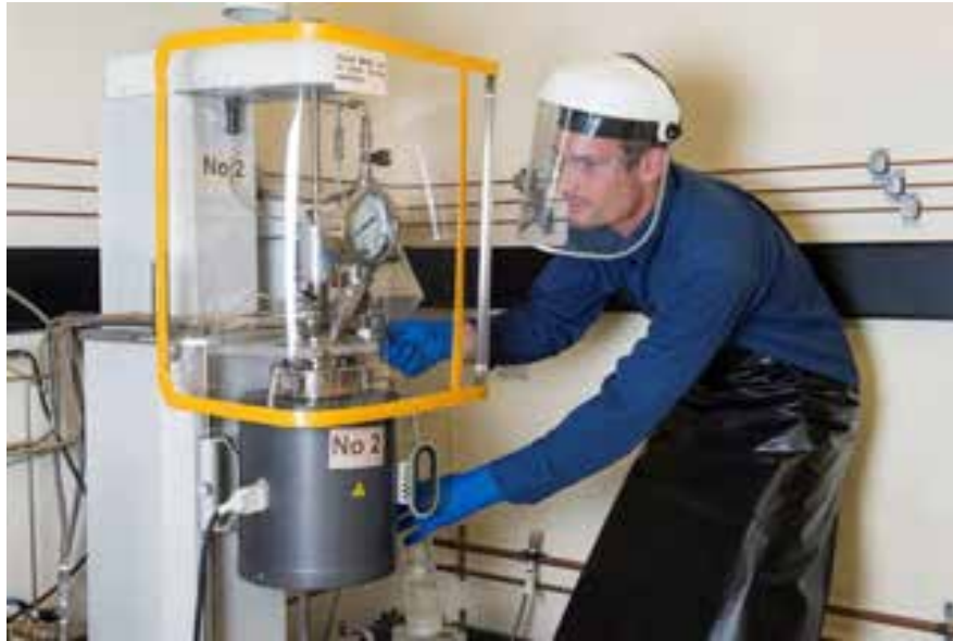
Figure D1 Example of autoclave equipment at ANSTO – high pressure acid leach (HPAL), pressure oxidative leach (POX) and caustic conversion – up to 2 L scale, number of materials of construction options
