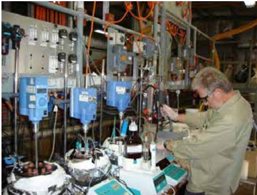
Figure A4 Uranium leach circuit – pH controlled acid leach
