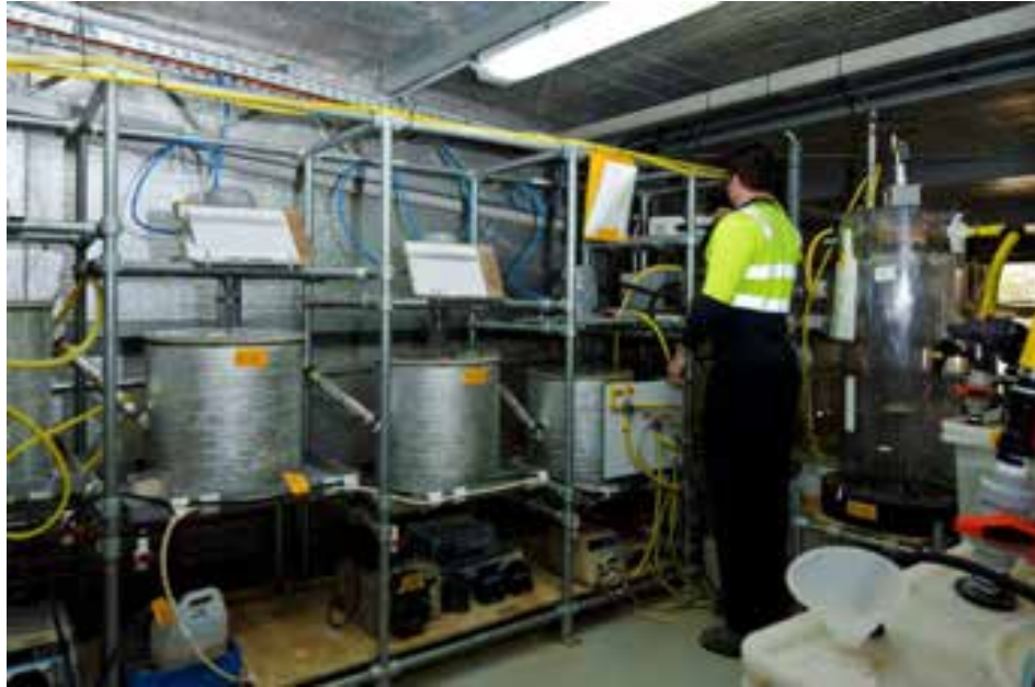
Figure B1 RE leach circuit – pH controlled acid leach – at ANSTO
