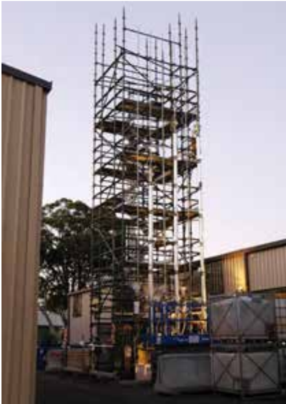
Figure H3 Pulsed column demonstration plant designed / built by ANSTO for uranium at ANSTO
