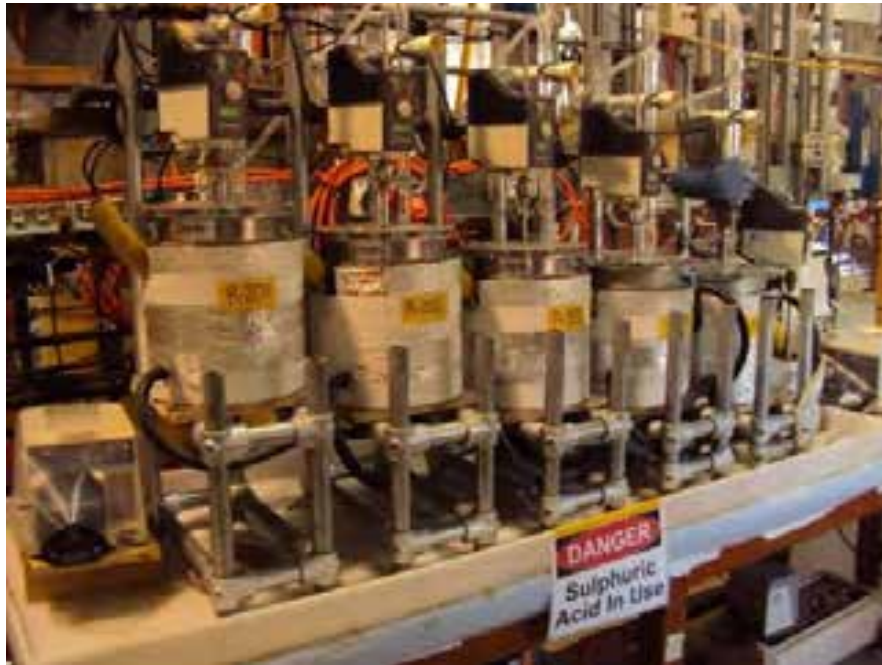
Figure C1 Lithium ore leach circuit at ANSTO
