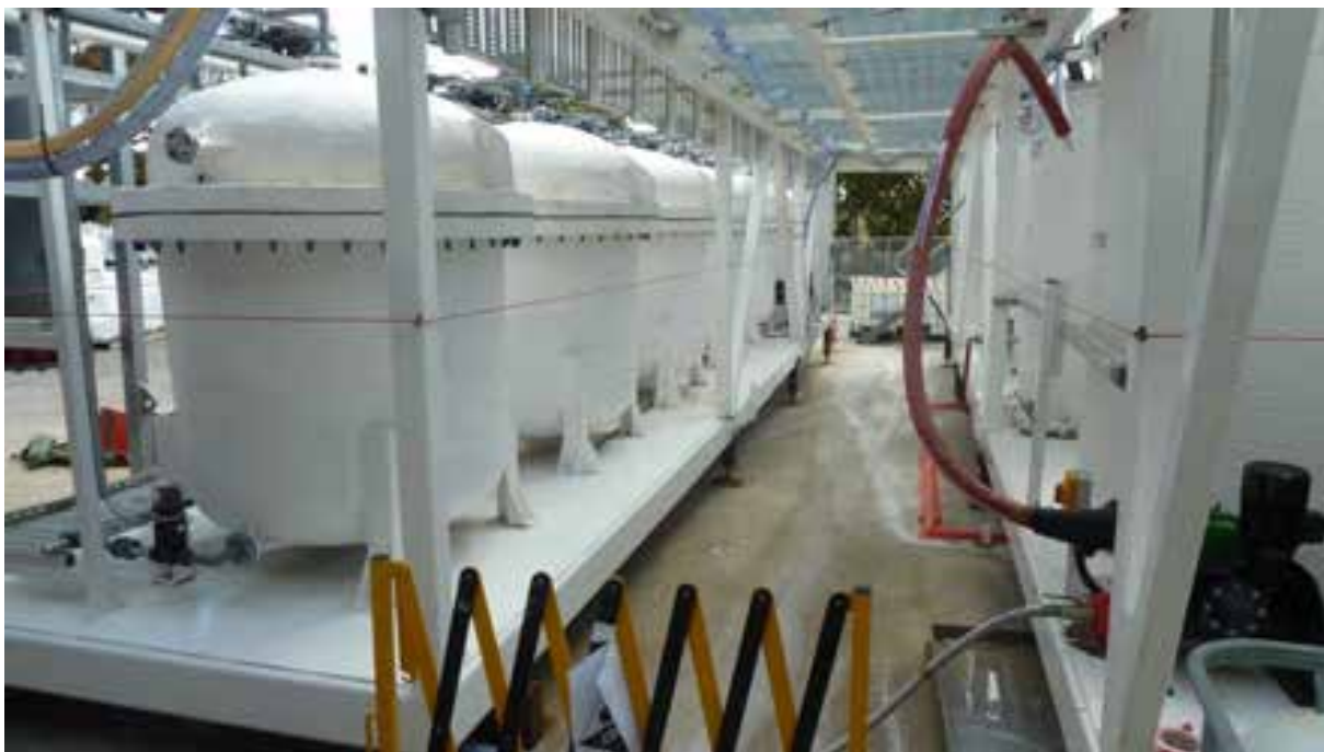
Figure C8 Brine processing demonstration plant at ANSTO – lithium carbonate precipitation circuit
