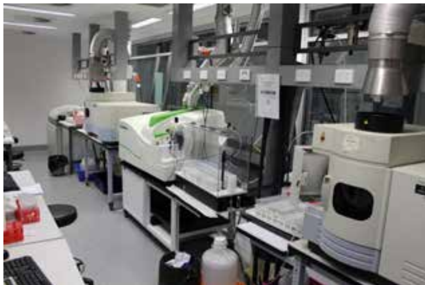
Figure G3 Inductively Coupled Plasma Optical Emission and Mass Spectrometers (ICP-OES x 2 and ICP-MS x 2)
