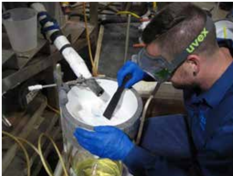
Figure C6 Lithium carbonate chemical concentrate production at ANSTO
