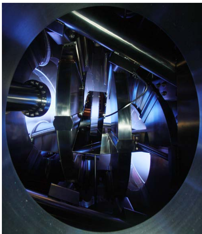
Figure 4: A section of the H-1 magnetic field coil structure needed to generate the helical magnetized plasma (blue emission)
