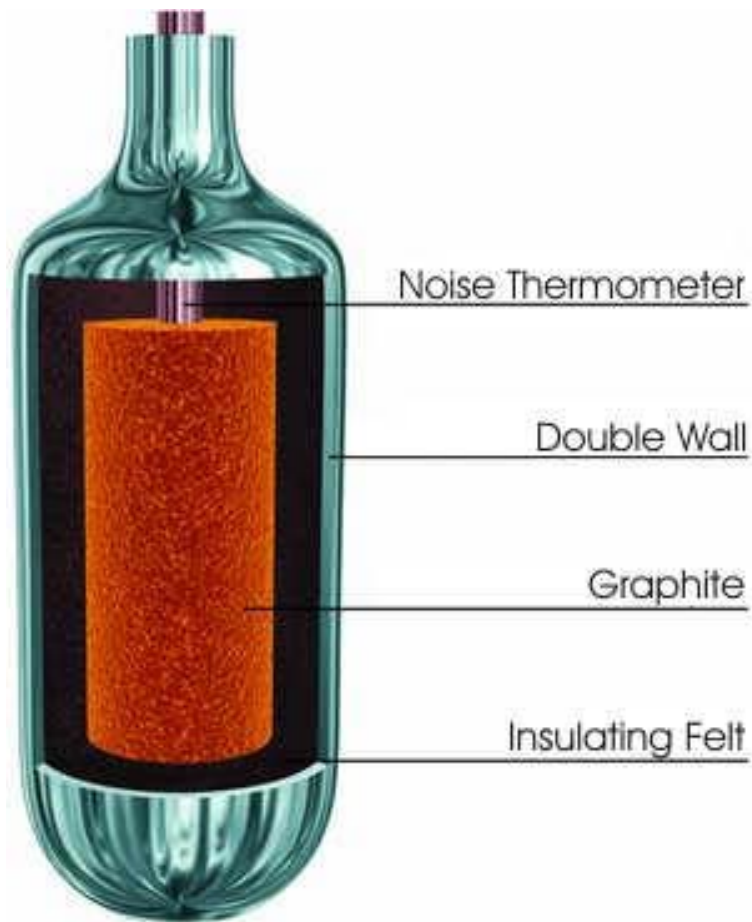
Fig. 16 Schematic diagram of the hot neutron source at FRM-II
